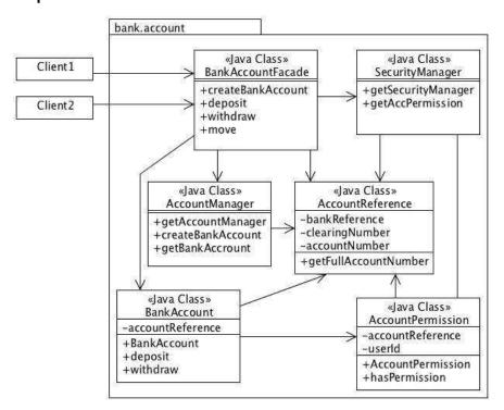
Consider the graphics above, where the Client classes makes calls to the BankAccountFacade class. The Facade class uses the classes AccountManager, SecurityManager, AccountReference and BankAccount to perform the appropriate actions. By using the Facade pattern we decouple the client code from the implementation and security details when performing tasks related to the bank account.
