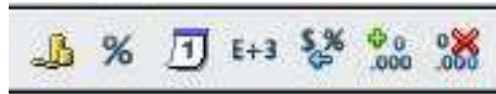
Figure 93: Number format icons. Left to right: currency, percentage, date, exponential, standard, add decimal place, delete decimal place.
