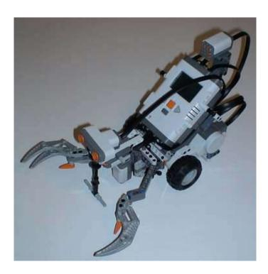
We also need the test pad with the black track that comes with the NXT set. The basic principle of line following is that the robot keeps trying to stay right on the border of the black line, turning away from line if the light level is too low (and sensor is in the middle of the line) and turning towards the line if the sensor is out of the track and detects a high light level. Here is a very simple program doing line following with a single light threshold value.
