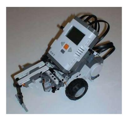
Connect the touch sensor to input 1 on the NXT.
