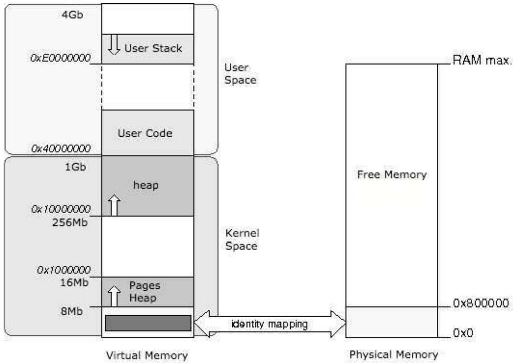
The kernel space in virtual memory, which is using 1Gb of virtual memory, is common to all tasks (kernel and user).
