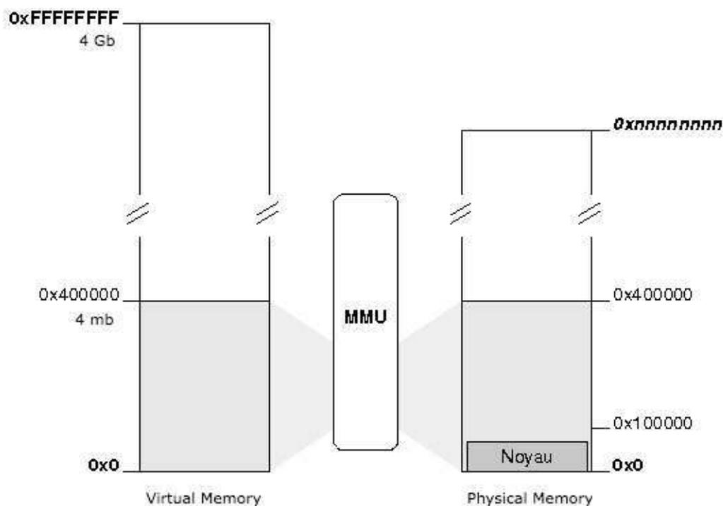
This model is simple: the first virtual memory page coincide to the first page in physical memory, the second page coincide to the second page on physical memory and so on ...
