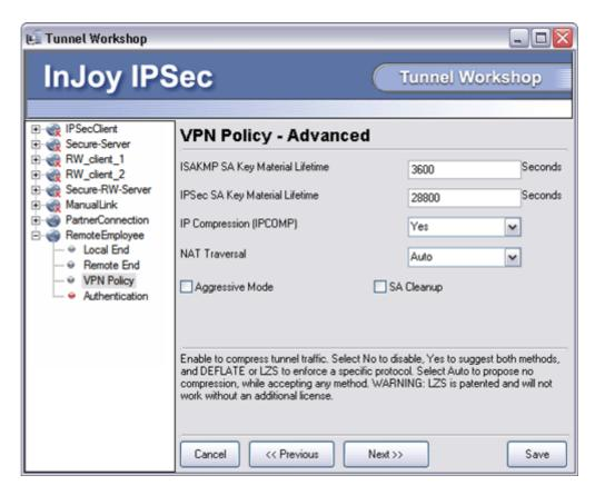
Because the employees use slow dial-up lines, it is helpful to mitigate the overhead imposed by IPSec. This is done using IP compression, which can at times significantly increase throughput. Aggressive mode is left disabled for this connection, since the employees will be using main mode negotiation.
