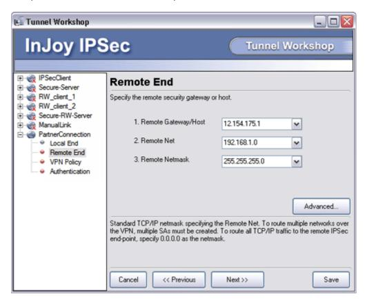
In the Remote End dialog, the network administrator enters the host address of the partner company's gateway, 12.154.175.1, as the remote host. The remote net and remote netmask are then set to 192.168.1.0 and 255.255.255.0, accordingly.
