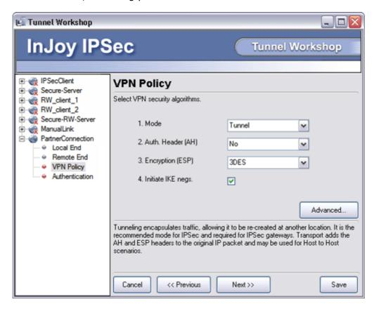
In the VPN Policy dialog, he configures for tunnel mode, without authenticated headers, using the more secure 3DES cipher and he selects this end-point can initiate IKE-negotiations.
