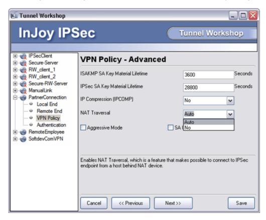
In the configuration files, the absence of a NAT-Traversal keyword for a particular security association indicates that NAT-T is enabled and will function as necessary (automatically). To explicitly disable NAT-T for a particular Security Association, set the value of the NAT-Traversal keyword to "No" as shown below:
