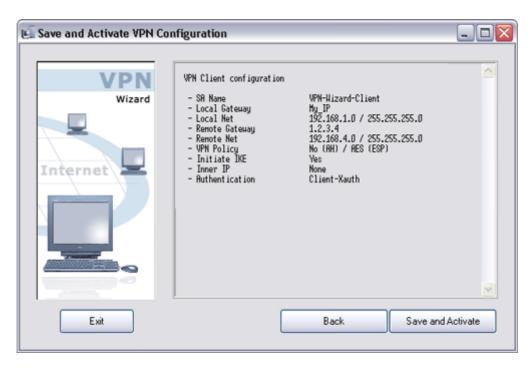
Once you click "Save and Activate", IPSec will enable your configuration and if you were setting up a VPN Client, a tunnel will be attempted set up with the remote VPN Server.
