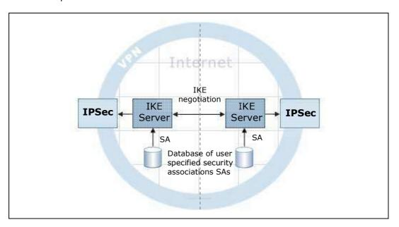
Above, the user-configured SA is provided to the IKE Server for negotiation with the remote IPSec end-point(s). Upon successful negotiation, the run-time SA is provided to the IPSec module, allowing it to apply packet transformation to all IP packets that match the SA
