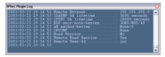
The IPSec Plugin Log, showing a new SA being installed for a remote user.
