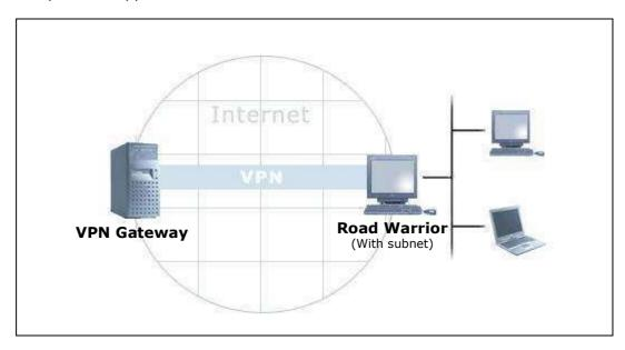
To properly utilize this support, the VPN Gateway **must** be configured with a common Road Warrior SA that defines a Remote Network of "appropriate proportions"; i.e. with enough addresses to allow the remote Road Warriors to define their own subnets within this "master network".
