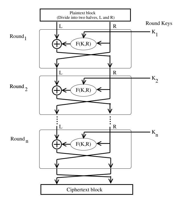
Figure 2: The Feistel Structure for symmetric key cryptography (This figure is from Lecture 3 of "Lecture Notes on Computer and Network Security" by Avi Kak)
