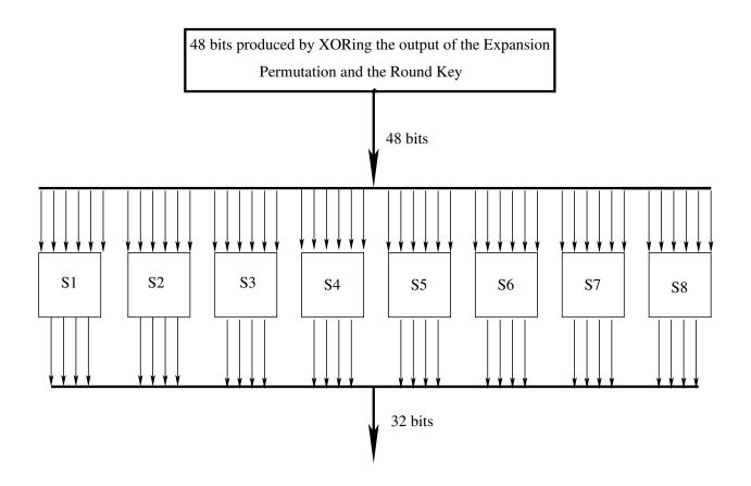
Figure 5: The 48 bits coming out of the expansion permutation are first XORed with the round key and then, as shown, fed into the 8 S-boxes of DES. (This figure is from Lecture 3 of "Lecture Notes on Computer and Network Security" by Avi Kak)
