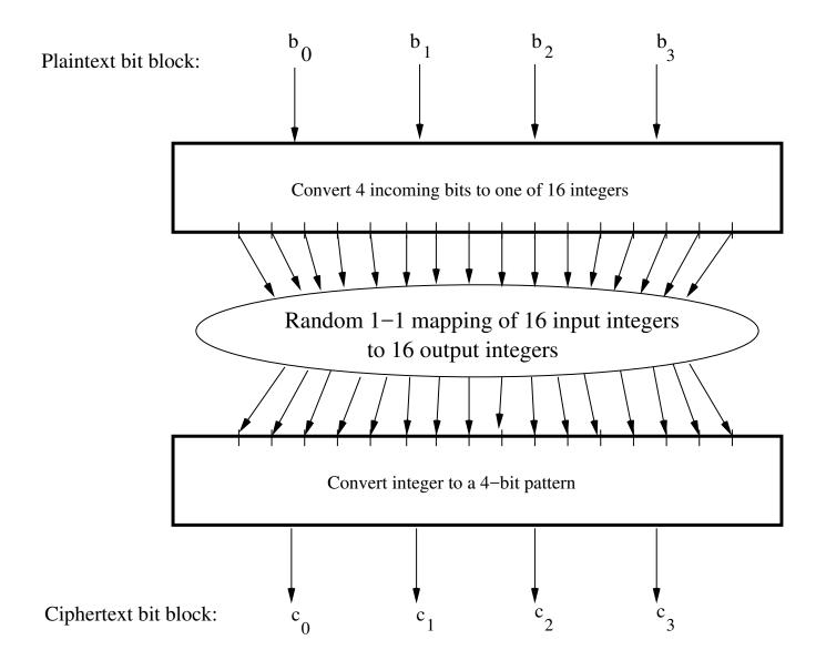
Figure 1: The ideal block cipher when the block size equals 4 bits. (This figure is from Lecture 3 of "Lecture Notes on Computer and Network Security" by Avi Kak)
