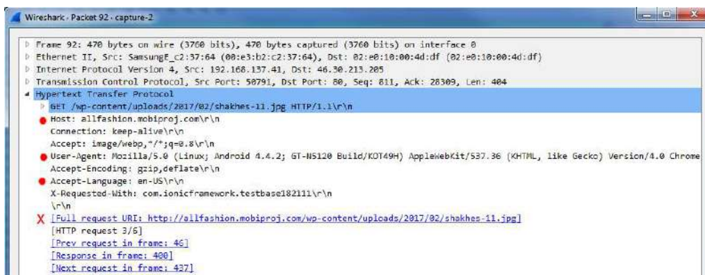
Figure 31. MiM Inspecting a single image request packet
