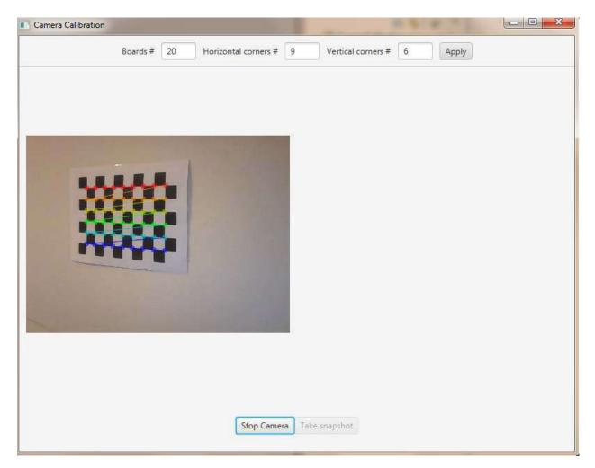
We should take the set number of "snapshots" from different angles and depth, in order to make the calibration.
