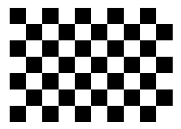
The reason why we use this image is because there are some OpenCV functions that can recognize this pattern and draw a scheme which highlights the intersections between each block. To make the calibration work you need to print the chessboard image and show it to the cam; it is important to maintain the sheet still, better if stick to a surface. In order to make a good calibration, we need to have about 20 samples of the pattern taken from different angles and distances.
