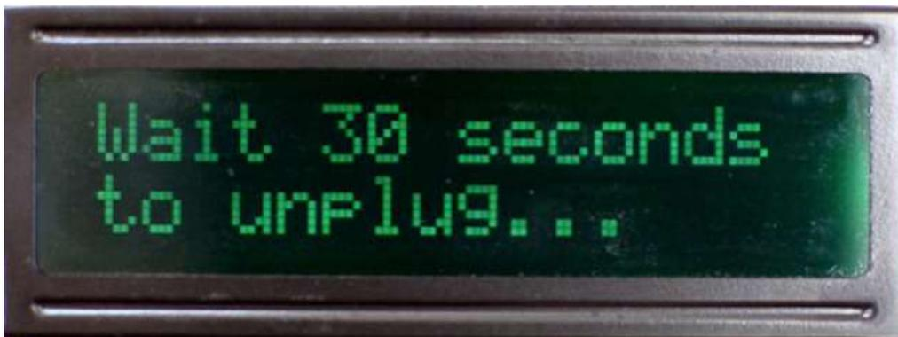
At this point, the Raspberry Pi will run through its shutdown routine and halt all processes. You'll need to wait up to 30 seconds before unplugging and/or restarting your Pi.
