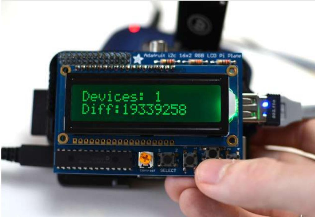
The LCD Plate's buttons can be used to adjust the info displayed and control the backlight.
